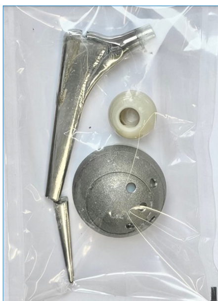
Figure 1: An 85-year-old lady sustained a periprosthetic fracture of the proximal femur with a broken stem. Before revision hip replacement, she requested to keep her removed implants. Post-operatively, the removed implants were washed and given to the patient in a clear sample bag.
