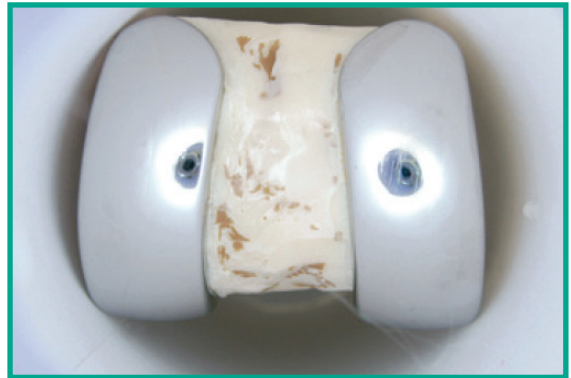
CoCrMo in TKA design with visible scratches after PE-Wear simulation under bone cement particle contamination. 10
