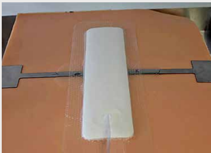
Figure 5: Experimental setup with Syndaver tissue model. The incision was closed with running stitch using 2-0 non-dissolvable suture 5mm apart. Dressing was applied on top of the incision model.
