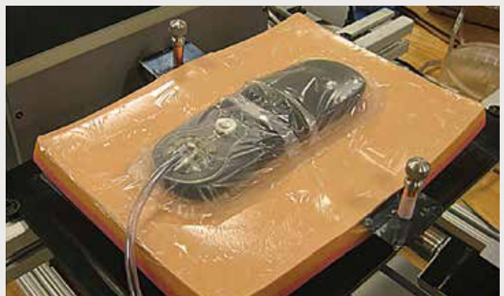
Figure 3: Incision bench model configured for horizontal extension-force testing with negative pressure wound therapy dressing applied.
