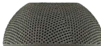
Fixa Ti-Por ® cup before and after deformation test
